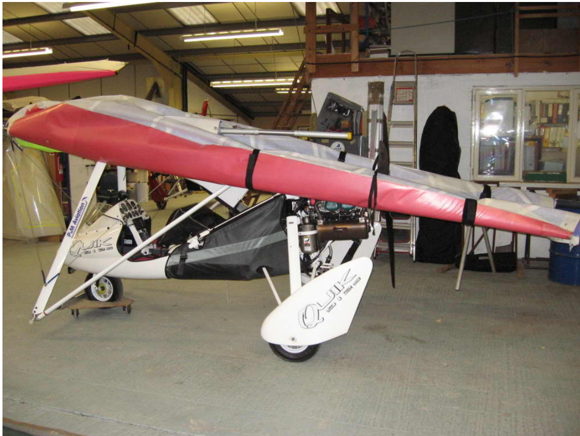
Fold configuration 2 – side view. The nosewheel skate allows movement in the hangar.
