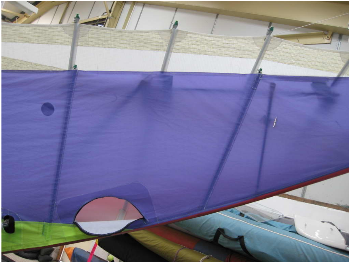
Rigging stage 12 – correct positioning of washout rods.
